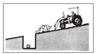
Pile dirt on the high side for easier backfilling on a slope.
